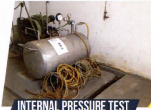
INTERNAL PRESSURE TEST
